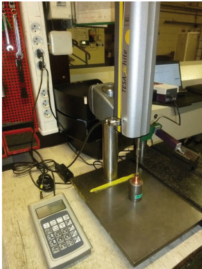
Measuring the sleeve of a crimping tool using the TESA-μHITE measuring station
