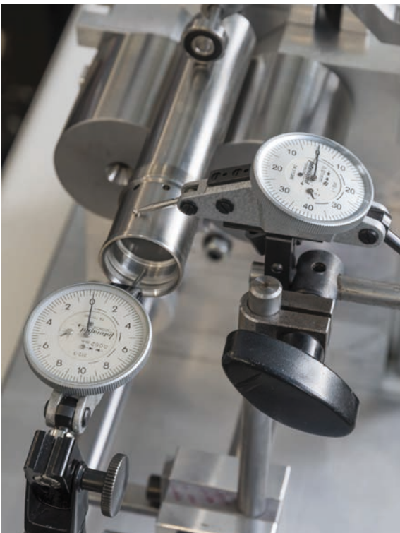
Measurement of radial runout errors of a workpiece on a measuring bench
