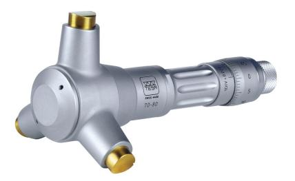
Internal micrometers from the TESA IMICRO range offer a market advantage. Their unique technology offers a precise and quick measurement of cylindrical bores. In fact, the drive of the measuring anvils via the spiral measuring cone allows linear control of the displacement of the instrument. In addition, the ratchet allows a constant measuring force.
