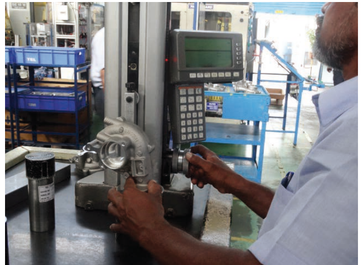
Two-dimensional inspection of bore positions in machined housing
