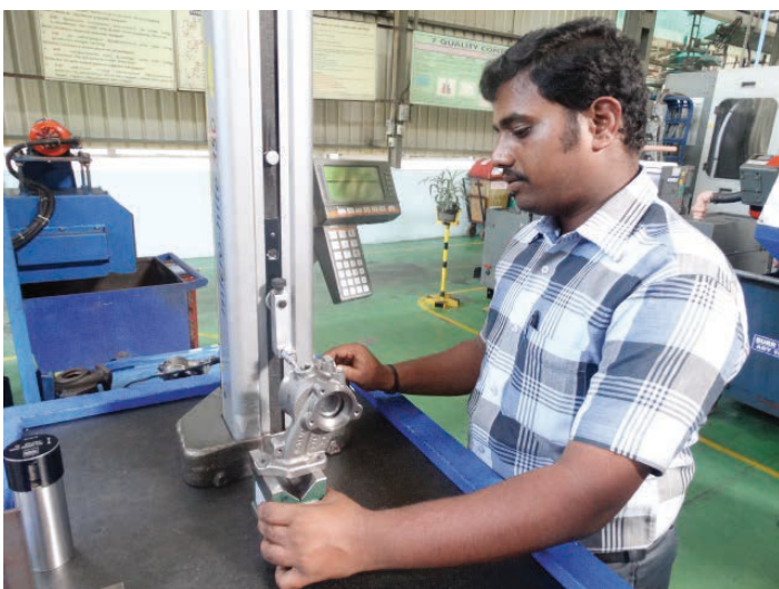
Bore measuring in machined housing mounted on a V-block
