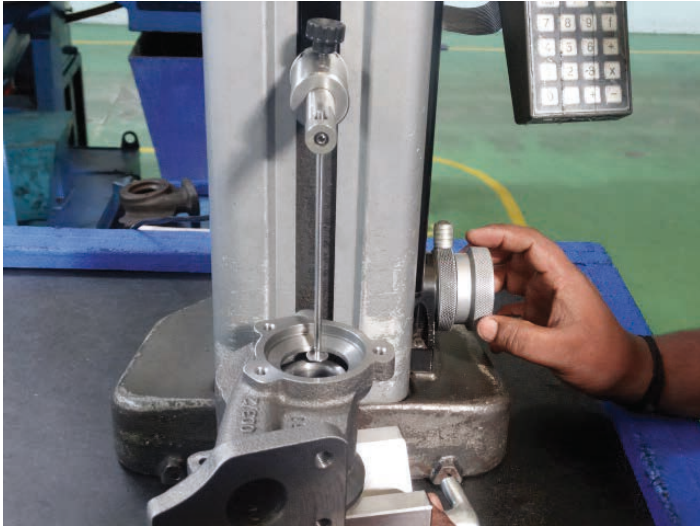
Depth measuring in machined housing mounted on a V-block
