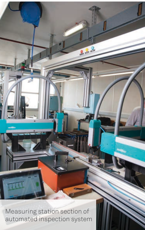
TESA blade inspection fixture and 2 BPX 44 boxes
