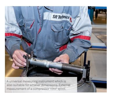
SR Technics is impressed by the versatility, flexibility, stability and low maintenance requirements of the TESA UNIMASTER. The specialists agree that the portable measuring tool always allows them to meet the necessary tolerances quickly and precisely. It is easy to use and, therefore, produces reliable results in the case of measurements taken both horizontally and vertically.
