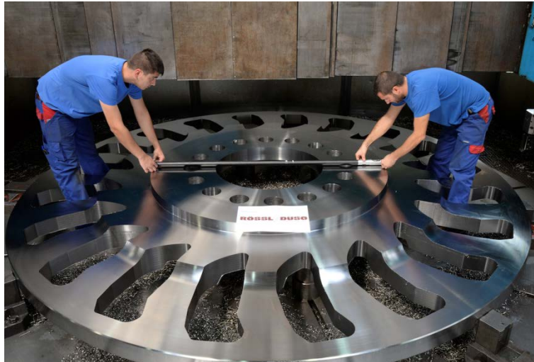
TESA UNIMASTER used by Rössl & Duso for measurement of a Pelton turbine
